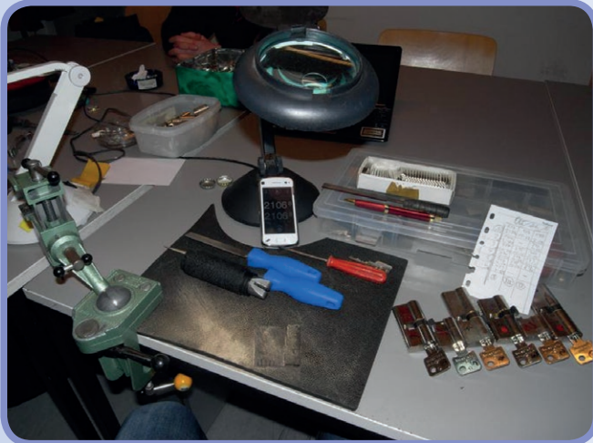
A work station used for the impression technique. The most important tools are the files and the handle. Especially high quality files with a Swiss cut 3 offer good impression marks..
