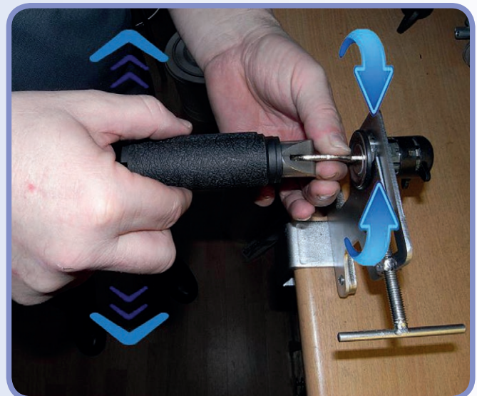
With the impression technique the fixed key is turned to the right or left in order to block the pins. By then swinging the key up- and downwards impression marks are generated on the key.
