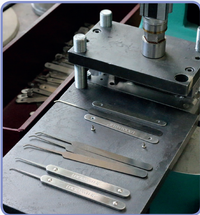
Finished cut handpicks are riveted with moulded recess handle.
